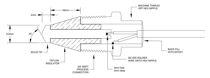
CONDUCTIVITY PROBE GROUNDED ON THE THREAD TEFLON INSULATOR
